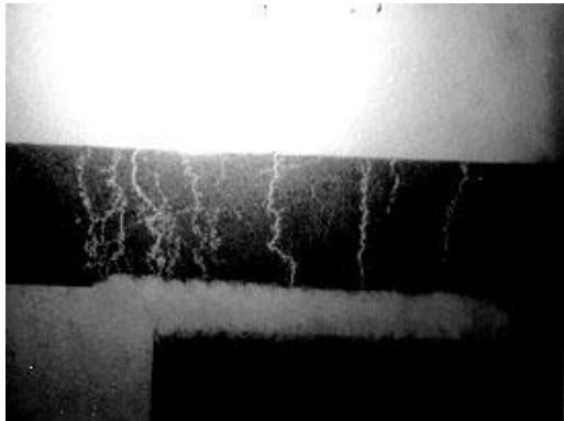
Fig. 8. Vicinal view of ESD induced damage to a thin-film resistor network chip during ground testing [1].
