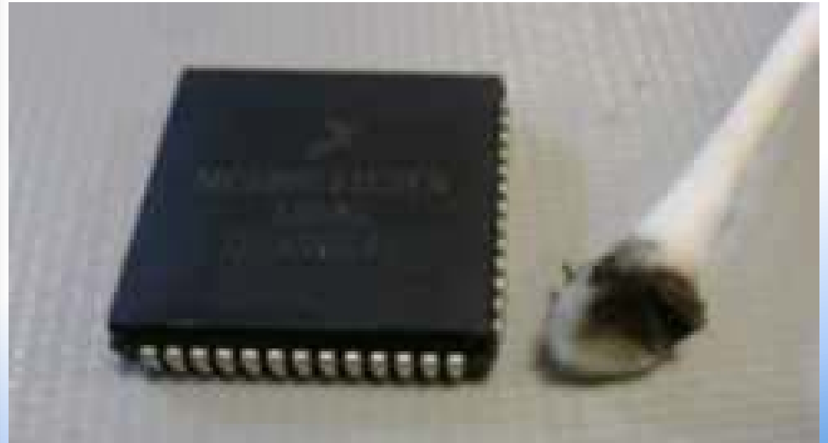
Acetone removes black from surface of part
