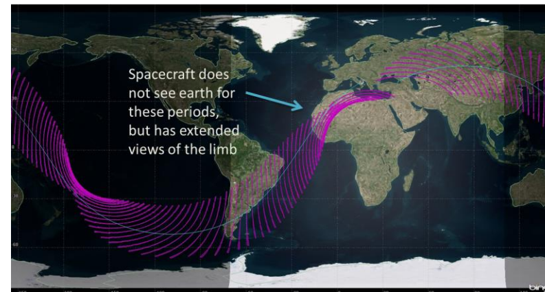
Radiometer Ground Track on Equinox
