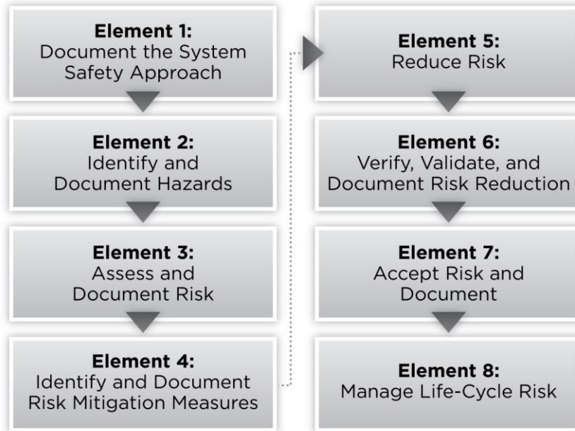
Figure 3 — MIL-STD-882E System Safety Approach
