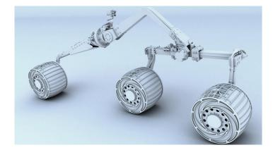
The rocker-bogie mobility system (the wheels surmounts the face of a vertical obstacle (rock) by having the center and rear wheels force the front wheels against the obstacle
