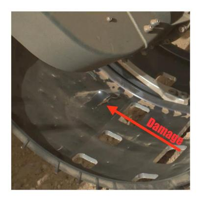
← Detail view of the inner surface of Curiosity's left front wheel on sol 411.
