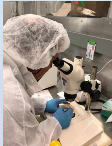
Visual enumeration of colony forming units after incubation at 32 °C for 24, 48, and 72 h
