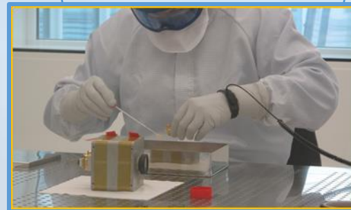
Verification – Swab of the ExoMars camera
