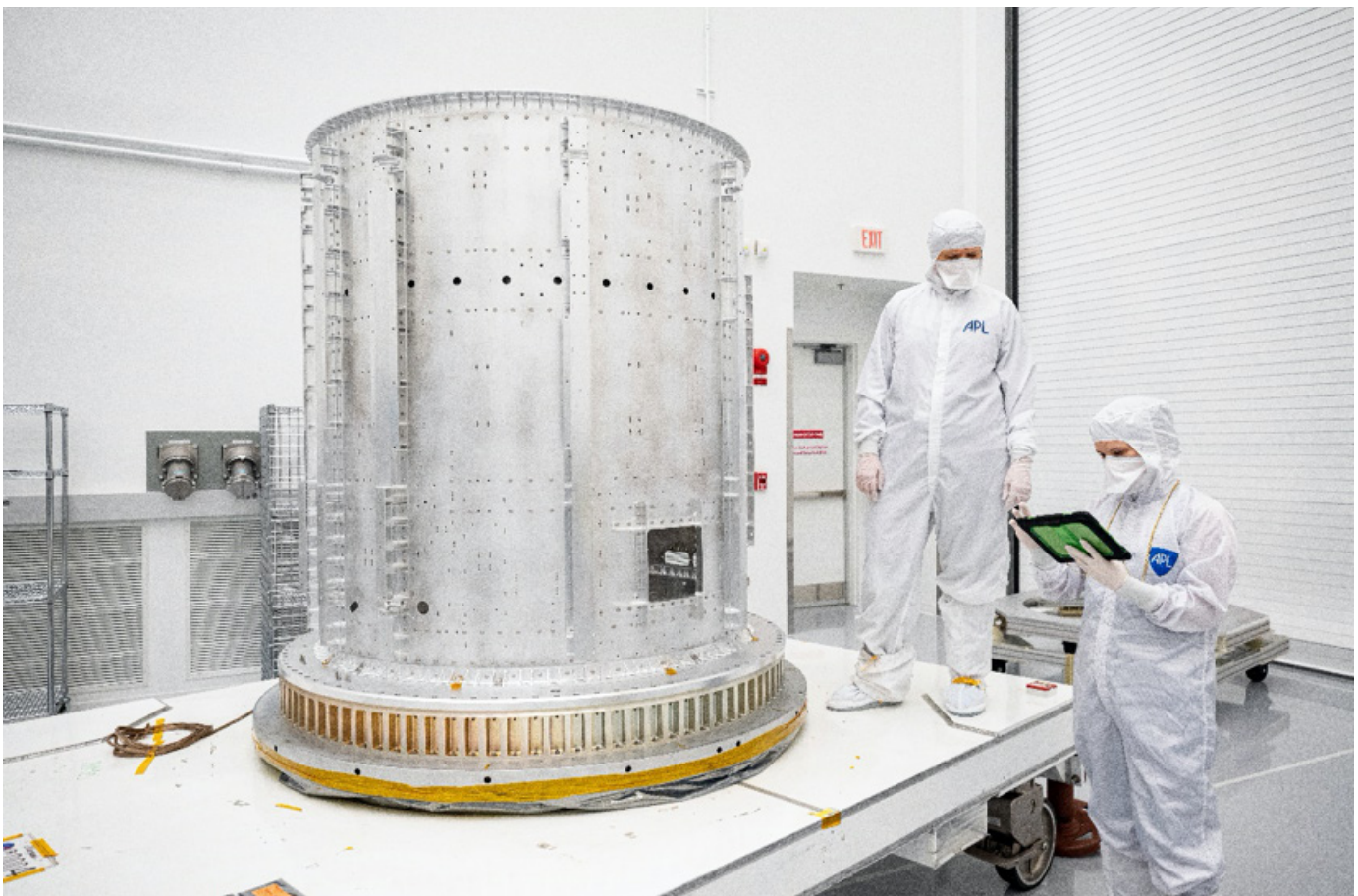
Applied Physics Laboratory (APL) engineers gowned and working on the upper cylinder of the Europa Clipper Spacecraft. Cleanroom garments include head and face covers, coverall, boots and gloves (photo provided by APL, used with permission)
