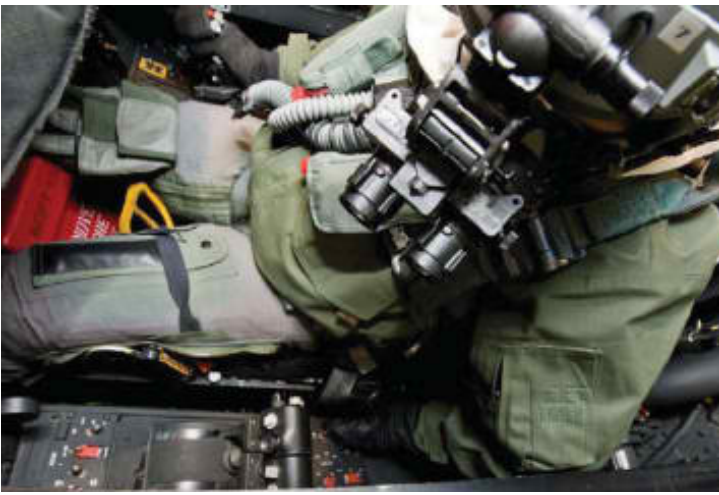
Figure 6. USAF Accident Investigation Board member wearing Category III cold weather gear and NVGs in F-22A cockpit.
