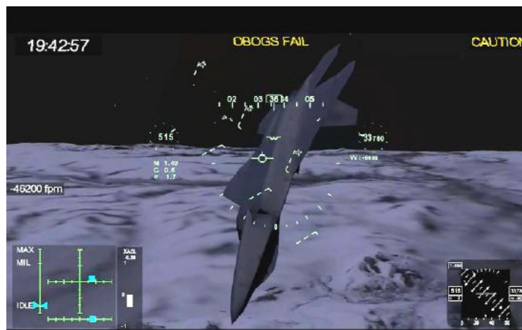
Figure 4. The MA inverted and plummeting with no control input from MP (no pressure to mask).
