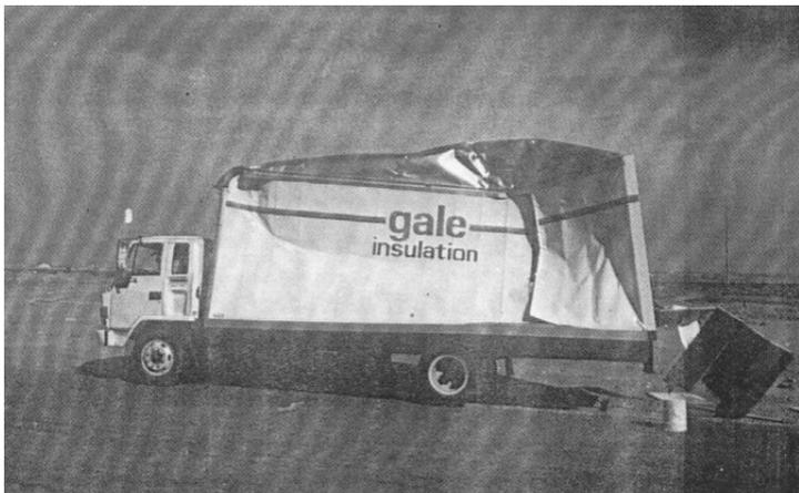
Figure 3. A truck displaying the effects of the shockwave from the second explosion. Source: United States Fire Administration.
