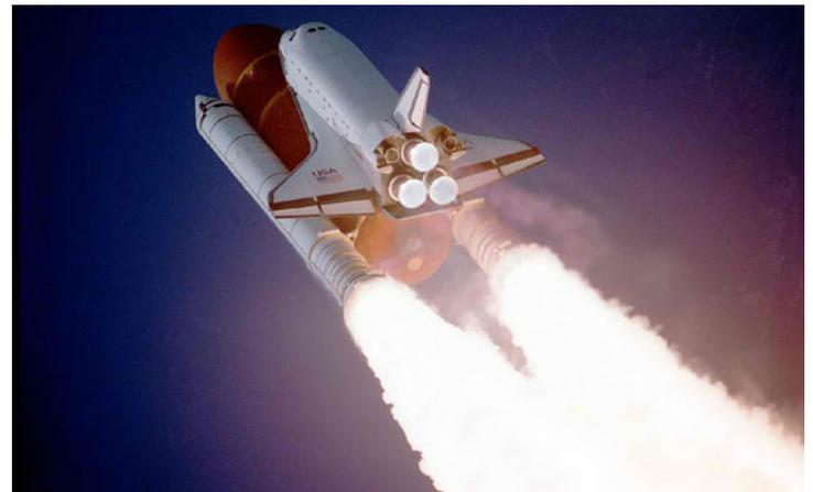
Figure 2. Each Space Shuttle SRB is loaded with approximately 550 tons of propellant. AP makes up 69.6% of the fuel (382.8 tons by weight) commonly referred to as Ammonium Perchlorate Composite Propellant (APCP). The remaining mixture comprises aluminum fuel (16%), iron oxide catalyst (0.4%), a polymer binder and secondary fuel (12.04%), and an epoxy curing agent (1.96%). NASA.
