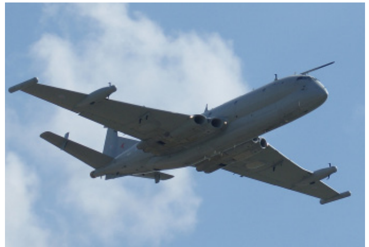
Figure 1: Nimrod in flight. Paired engines can be seen embedded in the wings, close to where the wings connect to the fuselage.
