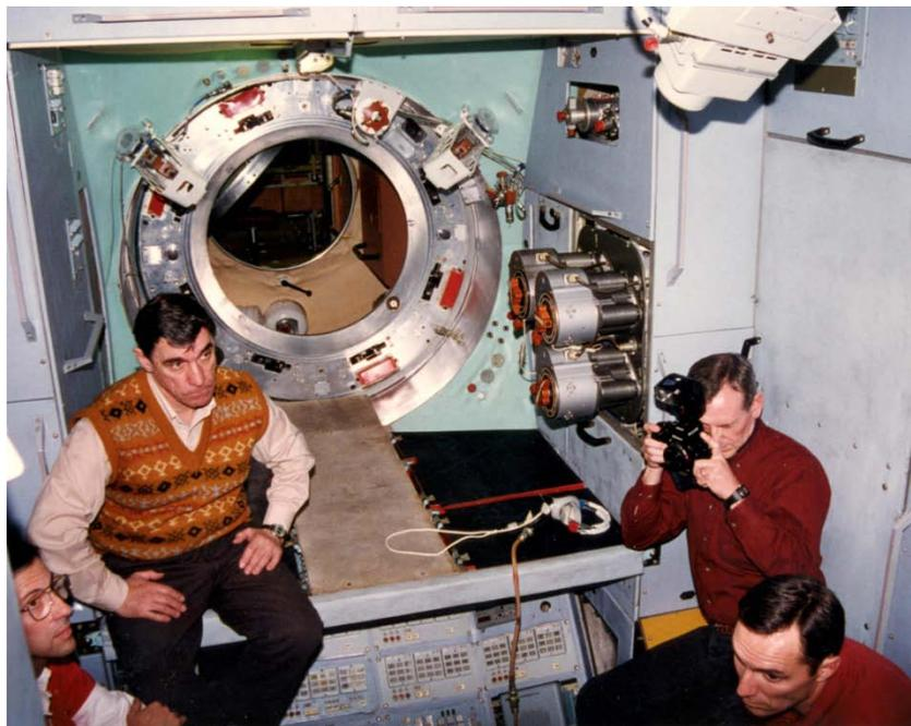
Figure 1: The solid fuel oxygen generator in *Mir's* *Kvant-1* module can be seen on the wall to the right of the hatch. When the fire ignited, it blocked the path through the hatch to the Soyuz. After the fire, new operating procedures dictated that only the SFOG in the base block would be used.
