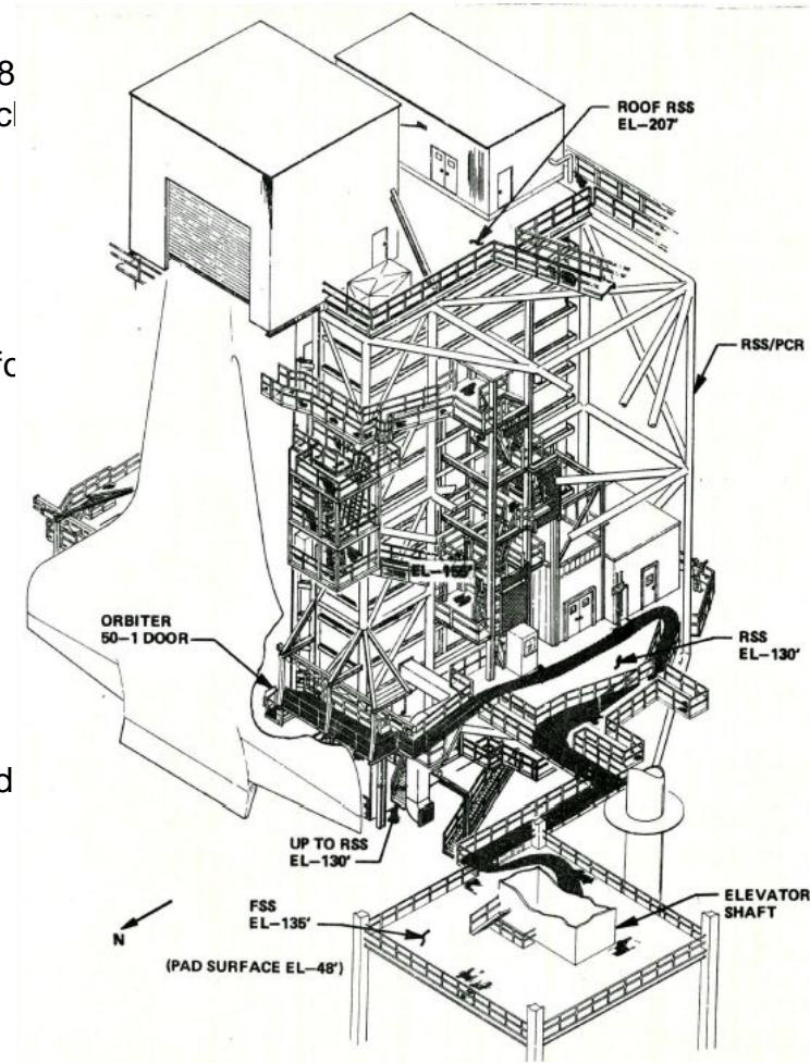
Path from elevator shaft to aft compartment
