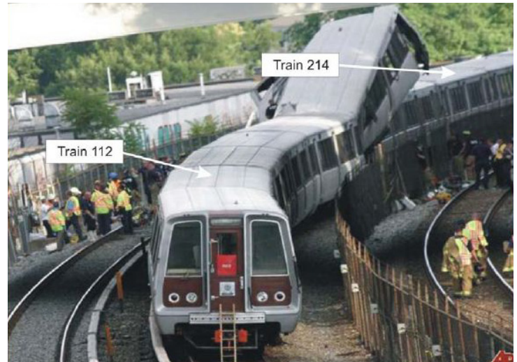
Figure 1: Train 112 was travelling at more than 40 mph when it crashed into stopped train 214.
