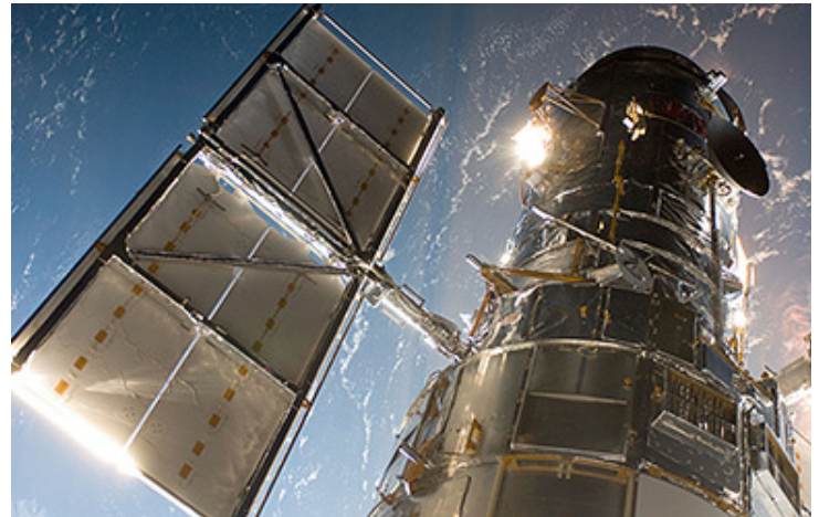
Figure 1: Hubble's vantage point in low-earth orbit allows it to collect a wider range of wavelengths than ground-based telescopes, and the images it captures are free from the atmosphere's distorting effects.
