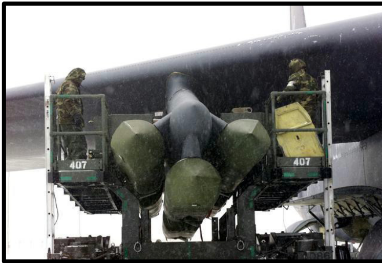
Top: A B-52 pictured on the runway at Minot AFB. Bottom: Airmen attach a pylon of AGM-129 Advanced Cruise Missiles to the wing of a B-52.
