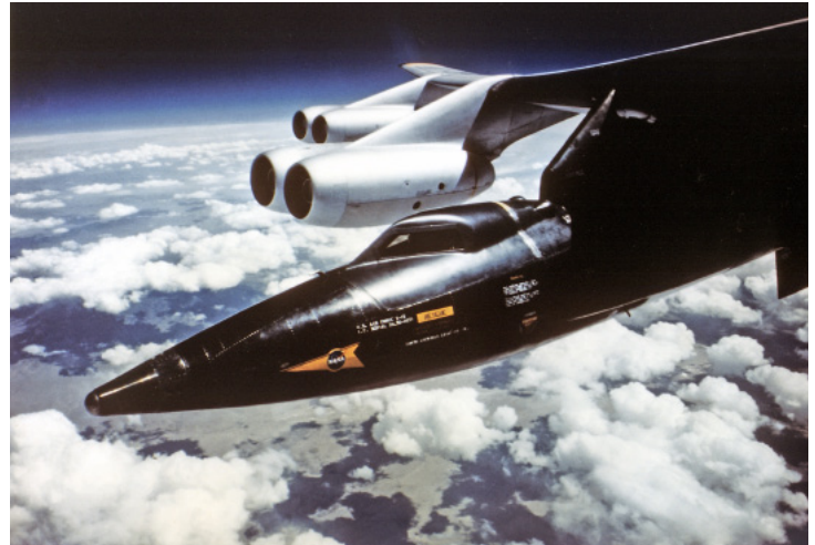
Figure 1: The North American X-15 rides beneath the starboard wing of a specially modified B-52A to launch altitude.
