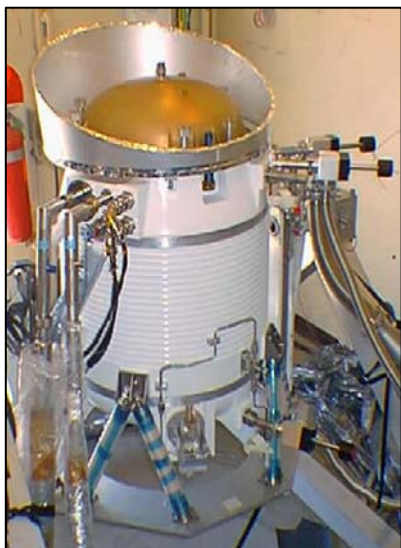
Figure 3: WIRE's cryostat cover (gold colored) shields the telescope and hydrogen tanks
