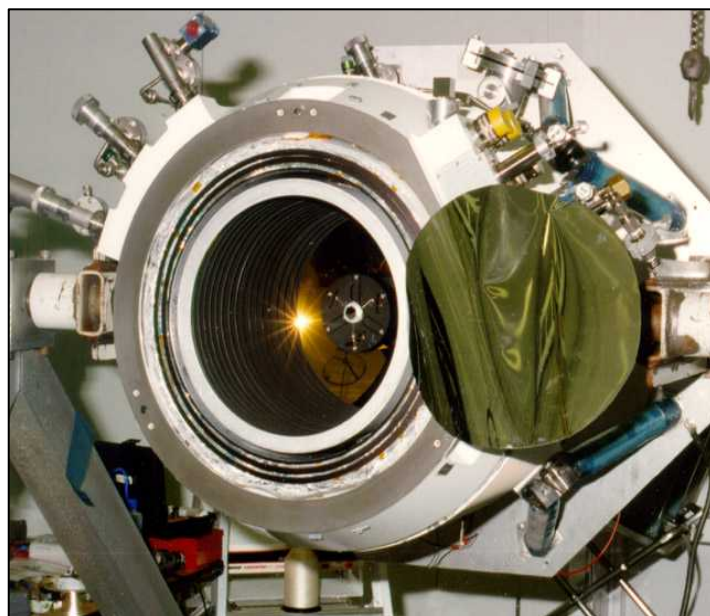
Figure 1: The open cover reveals WIRE's telescope in the center of the cryostat.
