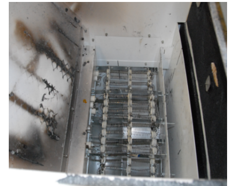
Heating element of the ECU where the filter fell and subsequently caught fire
