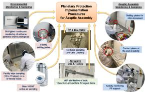
During the Mars 2020 aseptic assembly of hardware, stringent facility and hardware cleanliness monitoring was conducted using witness plates (settling and contact plates) to detect potential contamination. A total of 7,619 witness plates were deployed across 688 assembly activities, with plates incubated and monitored for microbial growth.
