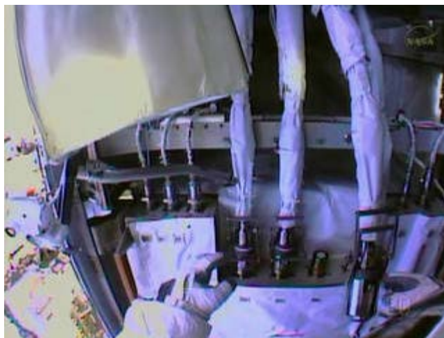
Spacewalker Rick Mastracchio works to disconnect the fluid lines from the degraded pump module in this view from the NASA astronaut's helmet camera.
