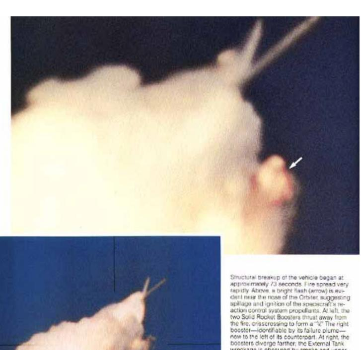
action control system propellants. At left, the two Solid Rocket Boosters thrust away from the fire, crisscrossing to form a "V." The right booster—identifiable by its failure plume—new to the left of its counterpart. At right, the boosters diverge farther, the External Tank wreckage is obscured by smoke and vapor. The Orbiter engines still firing, is visible at bollow center. boltom center.
