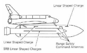
Drawing shows position of linear shaped charges and range safety command antennas on Solid Rocket Boosters and External Tank.
