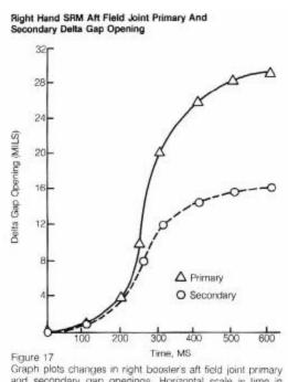
and secondary gap openings. Horizontal scale is time in milliseconds from ignition.
