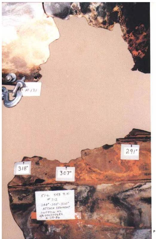
At upper left is the aft segment burn viewed from inside the casing; the lower photo is a closeup of the same section. The latter photo shows a hole (arrow) where the flame plume may have burned through the casing from the outside. At right is a composite view of the burn above and below the aft field joint.
