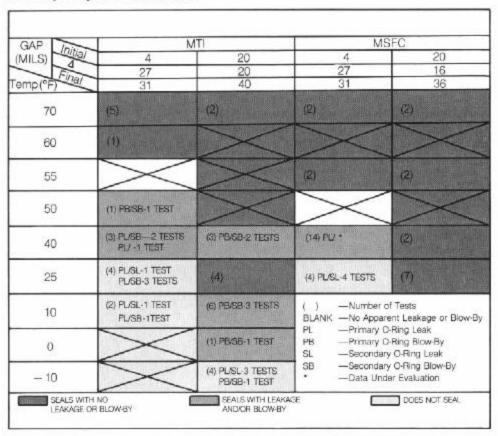
Figure 19. **Summary of Dynamic Test Results**. Table plots results of tests of .004 and .020 inch initial gap openings over the range of temperatures in left hand vertical column.
