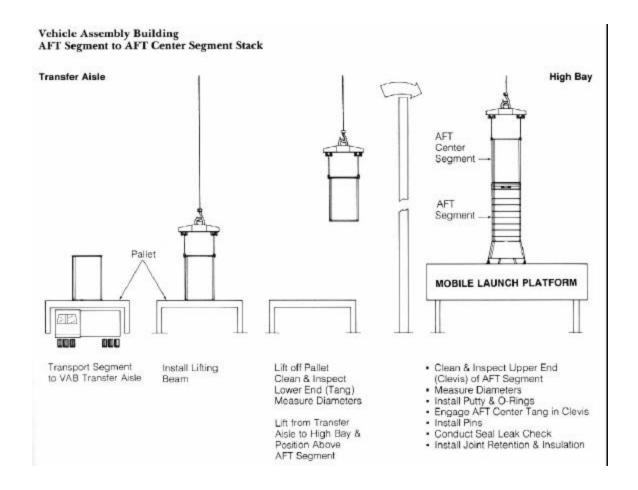
stacking interference. Taken across the 0180 degree axis, the tang diameter measurement exceeded the corresponding clevis dimension by +.512 inch. The maximum allowable tang to clevis difference is +.250 inch.
