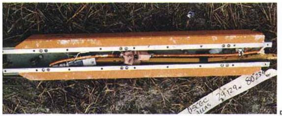
The lower photos show the range safety destruct charges in the External Tank. These charges were exonerated when they were recovered intact and undetonated.
