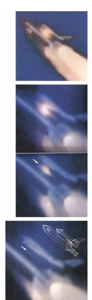
Camera views indicate the beginning of rupture of the liquid hydrogen and liquid oxygen tanks within the External Tank. A small flash (arrows above) intensified rapidly, then diminished
