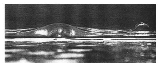
Pressure tests at 200 pounds per square inch of the Solid Rocket Booster joints produced bubbles in putty used to line the joints.
