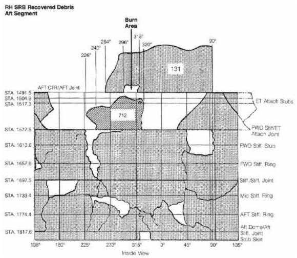
Drawing depicts pieces of right Solid Rocket Booster aft segment recovered. At top is piece of aft center segment.
