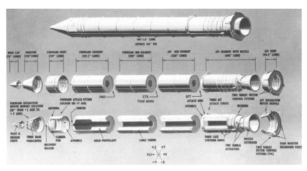
Figure 8. Solid Rocket Booster drawing at top is exploded in lower drawing to show motor segments and other elements at forward and aft ends of booster.
