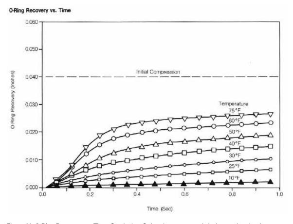
Figure 23. **O-Ring Recovery vs. Time**. Graph plots O-ring shape recovery in inches against time in seconds for a variety of temperatures. Note: Average O-ring Recovery at Various Test Temperatures During First Second After Load Release. Initial Compression of 40 Mils was Maintained for 2 hours.
