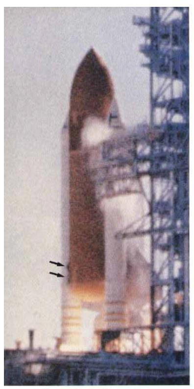
Multiple smoke pulls are visible in the photo above (arrows). They began at .836 seconds and continued through 2.500 seconds, occurring about 4 times a second. Upward motion of the vehicle caused the smoke to drift downward and blur into a single cloud. Smoke source is shown in the computer generated drawing (far right).
