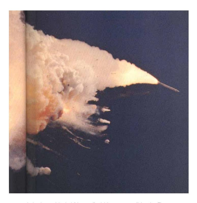
In the photo at right, the left booster (far right) soars away, still thrusting. The reddish-brown cloud envelops the disintegrating Orbiter. The color is characteristic of the nitrogen tetroxide oxidizer in the Orbiter Reaction Control System propellant
