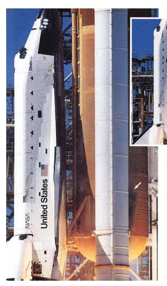
Immediately after solid rocket motor ignition, dark smoke (arrows) swirled out between the right hand booster and the External Tank. The smoke's origin, behavior and duration was approximated by visual analysis and computer enhancement of film from five camera locations. Consensus: smoke was first discernible at 678 seconds Mission Elapsed Time in the vicinity of the right booster's att field joint.
