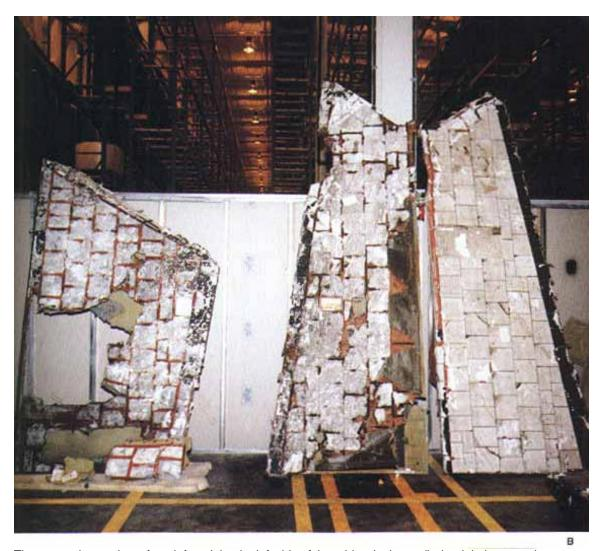
The upper photos show, from left to right, the left side of the orbiter (unburned), the right lower and upper rudder speed brake (both burned damaged) and left upper seed brake (unburned), confirmation that the fire was on the right side of the Shuttle stack.
