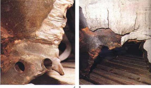
Photos I, J & K [clockwise]: Examined at Kennedy Space Center after their recovery from the ocean, these fragments show the extent of burn through the right hand booster's aft field joint. On the left page are sections of the aft center motor above the joint. On the right page are sections (inverted) of the aft motor segment showing burn-hole below the joint (bracket). Except for the interior views on lower left, the camera is viewing the parts from outside the casing.
