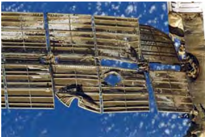
Figure 4: Mir solar array with collision-induced damage
