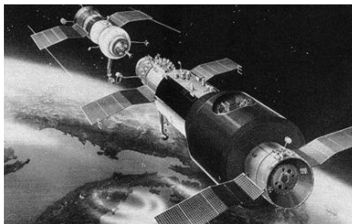
Figure 1: Artist's impression of a Soyuz spacecraft (left in picture) docking with Salyut
