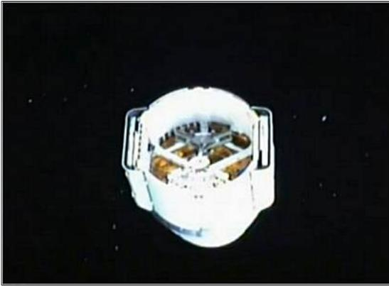
Dragon's helium pressurization problems occurred after main isolation valves were opened to release high pressure helium system. The helium passes through regulators that drop its pressure to a level that can be used into the hypergolic propellant tanks of the pressure-fed Dragon reaction control system. Check valves ensure that helium flows only into the tanks and that no propellant or helium flows back out.
