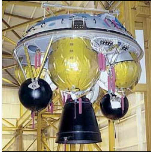
The upper stage for the Ariane 510 rocket is hoisted for attachment to the vehicle's cryogenic main stage in Kourou during pre-launch processing. Photo: Arianespace
