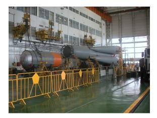
(HTTP://WWW.SPACESAFETYMAGAZINE.COM /2011/09/09/ROSCOSMOS-IDENTIFIES-CAUSE-OF-SOYUZ-FAILURE/PICTOO01/) HORIZONTAL ASSEMBLY OF A SOYUZ CORE BOOSTER WITH THIRD STAGE (CREDITS: ROSCOSMOS).
