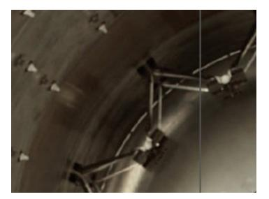
However, the flight telemetry does not fully support a "straightforward failure" of a loose helium bottle bur: ^ :r second stage tank.
