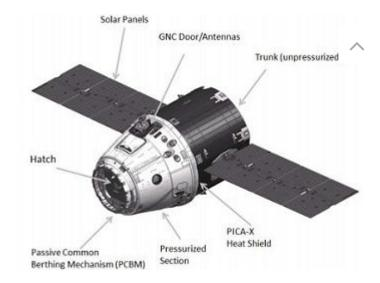
Dragon is a 5.9-metre (19.3-foot) long spacecraft, which has a diameter of 3.66 meters (12 feet), and is capable of carryir to 3,310 kilograms (7,296 lb) of cargo to the International Space Station. It can carry pressurized cargo to the ISS in a 2.<sup>o</sup> metre (9.5-foot) long capsule, which also provides 2,500 kilograms (5,500 lb) of downmass for returning supplies to Ea
