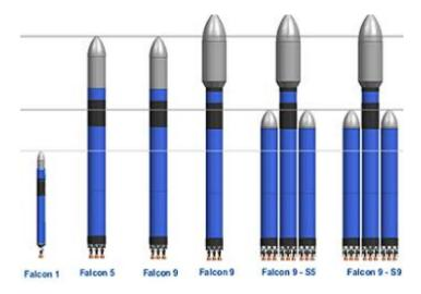
Falcon 1 and Falcon 9 were originally to have been joined by a third rocket, the Falcon 5. This was similar in design to th Falcon 9, however optimized for smaller payloads, with only five first stage engines.
