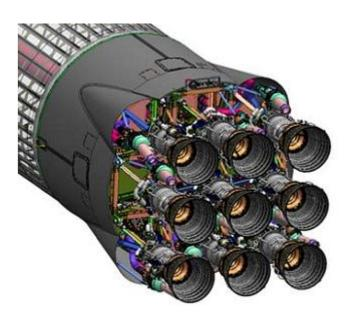
The Falcon 9 which launched CRS-2 is a two-stage vehicle. T first stage is powered by nine Merlin-1C engines arranged ir 3 square. A single vacuum-optimized Merlin-1C propels the second stage. Both stages burn RP-1 propellant, using liquid oxygen as an oxidizer.
