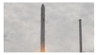
The command to ignite the first stage engines will be issued three seconds before liftoff, and when the countdown reach zero the Falcon 9 will begin its ascent into orbit for its fifth mission.
