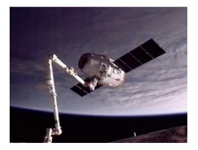
Dragon C2+ successfully completed a series of rendezvous demonstrations on 24 and 25 May, the last of which culmin in its approach to within nine meters (30 feet) of the space station, where astronaut Donald Pettit captured the vehicle using the Canadarm2 remote manipulator system. Followi capture, the RMS was used to berth the Dragon spacecraft the nadir port of the Harmony module. Hatches between t spacecraft and the ISS were opened on 26 May.
