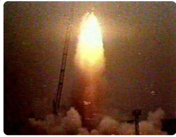
The escape tower propels Soyuz T-10A to dizzying altitudes and mind-numbing acceleration in the milliseconds after the abort. Cosmonauts Titov and Strekalov reportedly deactivated their cabin voice recorders because, "We were swearing!" Photo Credit: Joachim Becker / SpaceFacts.de
