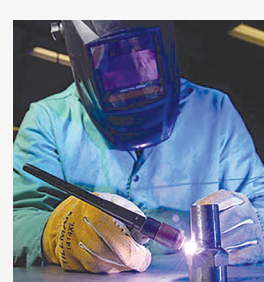
White Sands Test Facility: Carlos Sanchez performed a tig weld on a component with the proper Personal Protective Equipment (helmet, gloves and welding jacket) and proper work surface.
