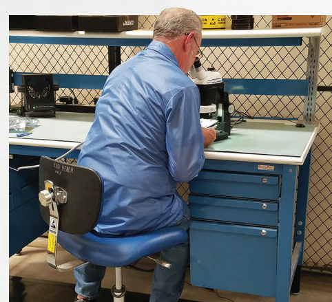
Armstrong Flight Research Center: LeRoy Marsh used an Electrostatic Discharge chair, mat and strap while inspecting a card as part of his Quality Assurance duties in the shipping and receiving area.
